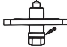
\* Do not lubricate the lower pivots of the THIRD WHEEL and INTERMEDIATE SECONDS WHEEL excessively. Be sure to observe the specified quantity.
