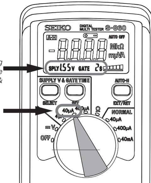
2. Read the measurement when a stable measurement is obtained.
