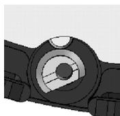
Ensure that the pins for dial fixing are securely engaged with the dial without any clearance.
