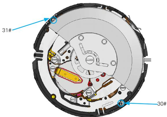
Rotation of the pins for dial fixing pins
