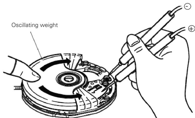
How to measure the current consumption for the CIRCUIT BLOCK alone
