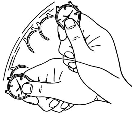
3. Within 3 minutes after swinging the watch, measure the voltage of the rechargeable battery in the same manner as in step "1" above.
