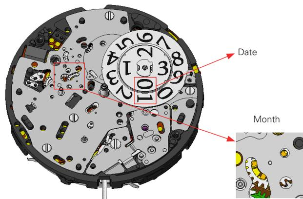
2. Pull out the SETTING STEM to the second click position, and turn the crown to set the 24H contact point as illustrated below (to correct the timing of date change).
