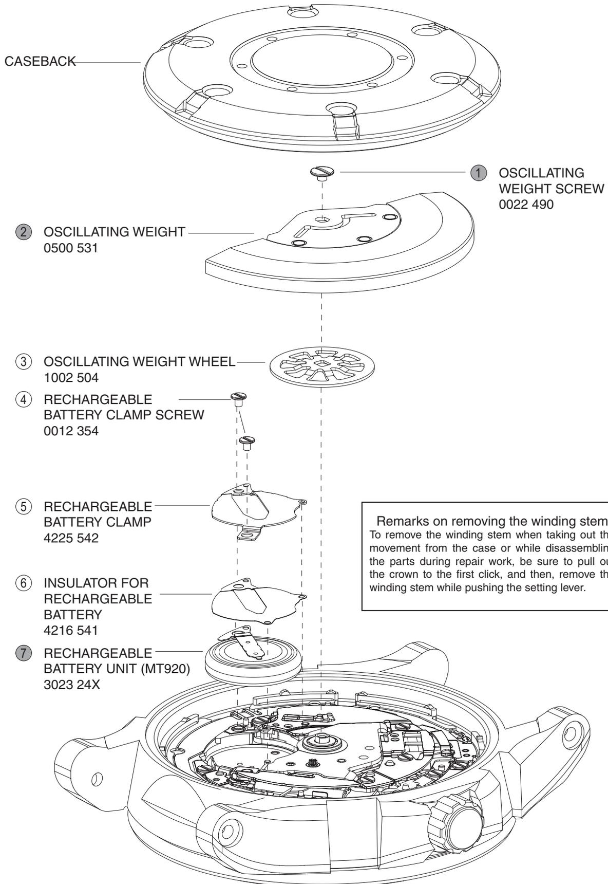
**Remarks on removing the winding stem**
