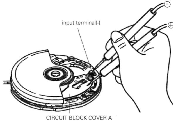
\* When measuring the current consumption using the SEIKO digital multi-tester (S-860), use the range of **40 μA** of **SUPPLY V (= 1.55 V)** & **GATE TIME (2 S)**
