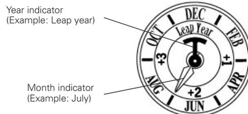
4. Turn the crown to set the month display hand to indicate the correct month. Then continue to turn the crown to set the date.
