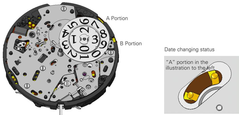
3. Keep the watch in this state when carrying out the installation of the hands in order of the 24-hour hand, month indicator, hour hand, minute hand and second hand.
